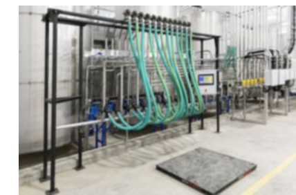
Small batches are accurately metered/ weighed with the same ICS ControlPro software as the larger bulk deliveries.
